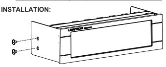
**Tools required:** Phillips head screwdriver Mount the product into a 5.25 inch drive bay of your computer chassis using the screws in the accessory bag.
